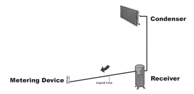
Systems using thermal expansion valves may have a receiver/tank on the outlet side of the condenser, designed to hold liquid refrigerant. When leaving the condenser directly or the receiver, the refrigerant remains a high pressure/high temperature liquid until it goes to the metering device. The line between the condenser and the metering device is also referred to as the **liquid line.**
