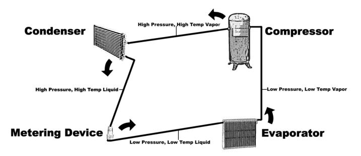
The **refrigeration process** is essentially the transfer of heat from one place to another. For example, in an air conditioning unit, the heat is removed from inside the building and is deposited outside the building. The vapor-compression refrigeration cycle is a repeating cycle consisting of four main components: the evaporator, compressor, condenser and metering device.
